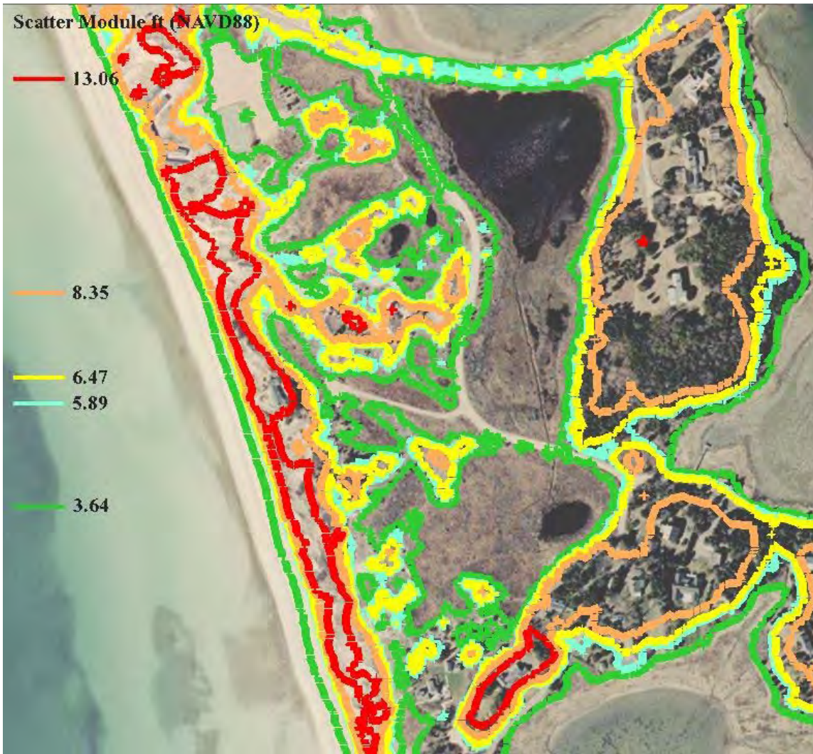
Figure 3-8. Contours showing the limiting elevations in the Little Neck Bay/Shrub Bog system for the 1-year (green), 3-year (cyan), 4-year (yellow), 10-year (orange), and 100-year (red) storm surge events.
