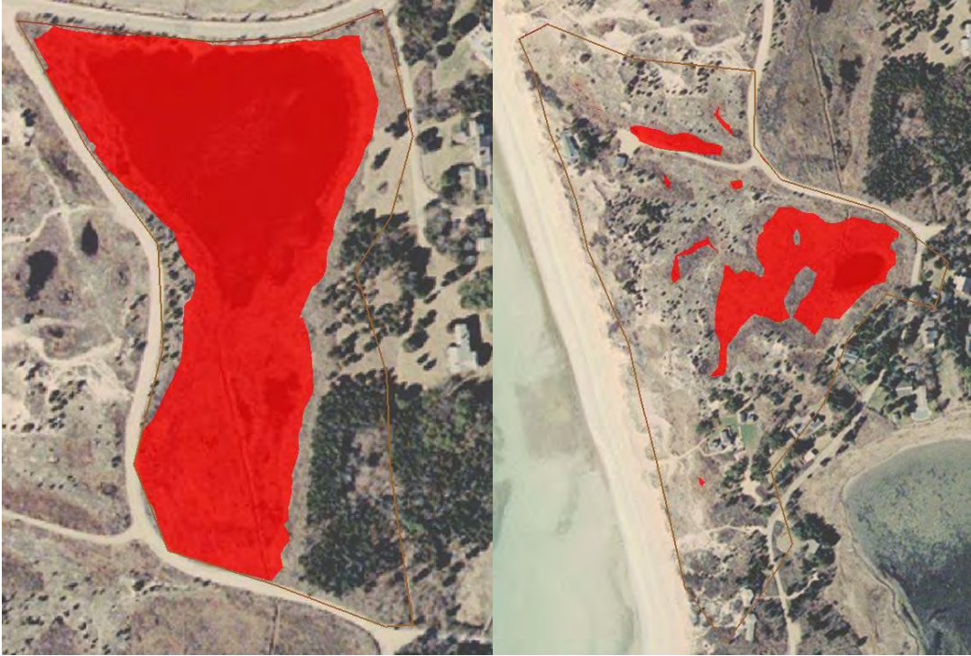
Figure 4-10. Extent of inundation for 3-year storm at Little Neck Bay (left) and Shrub Bog (right) for the culvert replacement and lowered invert elevation. (Note disconnected areas are not expected to be inundated and are an artifact of the elevation data).
