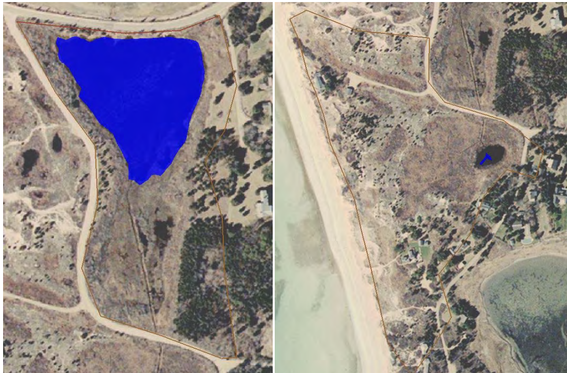
Figure 4-7. Extent of inundation at MLW at Little Neck Bay (left) and Shrub Bog (right) for the culvert replacement and lowered invert elevation.
