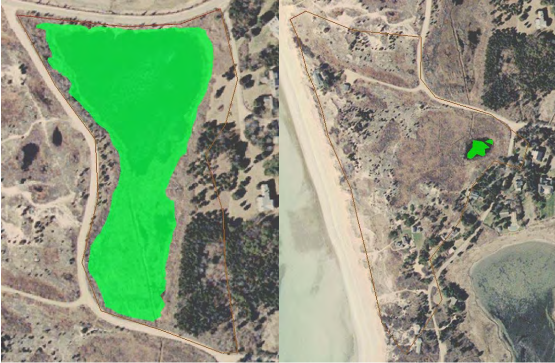
Figure 4-6. Extent of inundation at MHW at Little Neck Bay (left) and Shrub Bog (right) for the culvert replacement at the existing invert elevation.
