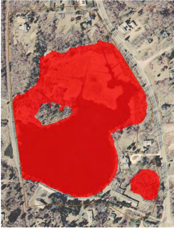
Figure 4-21. Extent of inundation for 3-year storm at Oyster Pond for the proposed box culvert with the shoals removed.
