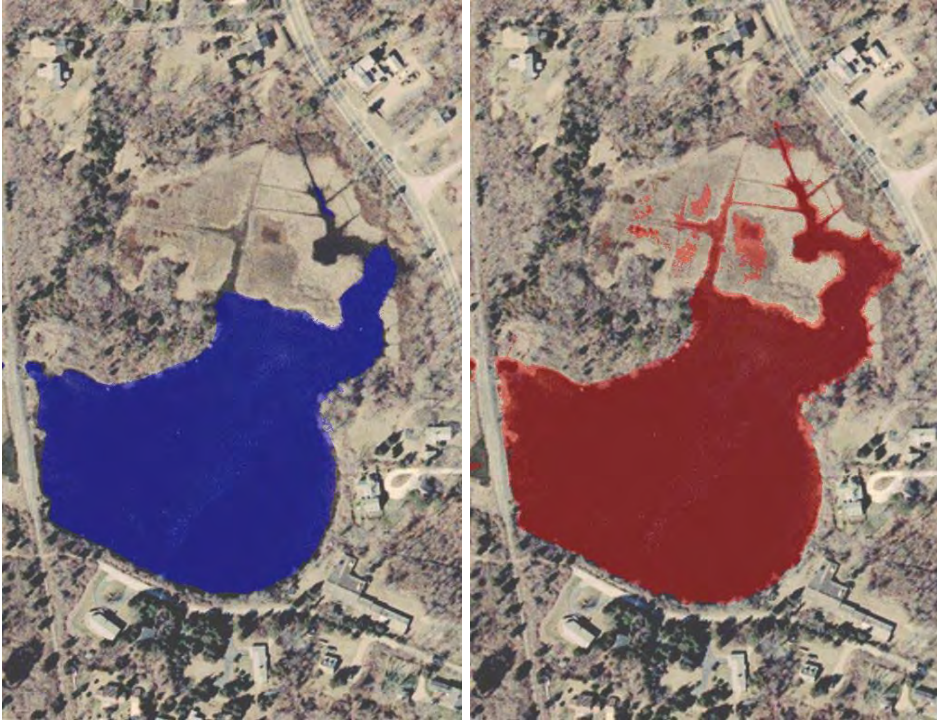
Figure 3-2. Extent of inundation in Oyster Pond at MLW (blue, left) and MHW (red, right) modeled WSE from Table 3.2.
