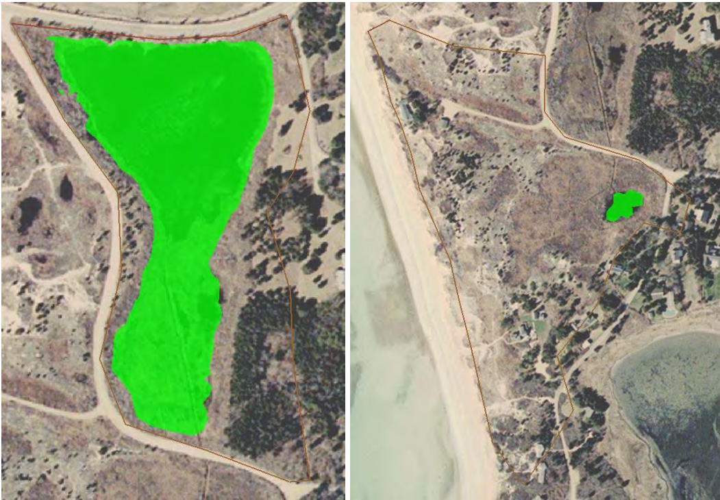
Figure 4-8. Extent of inundation at MHW at Little Neck Bay (left) and Shrub Bog (right) for the culvert replacement and lowered invert elevation.
